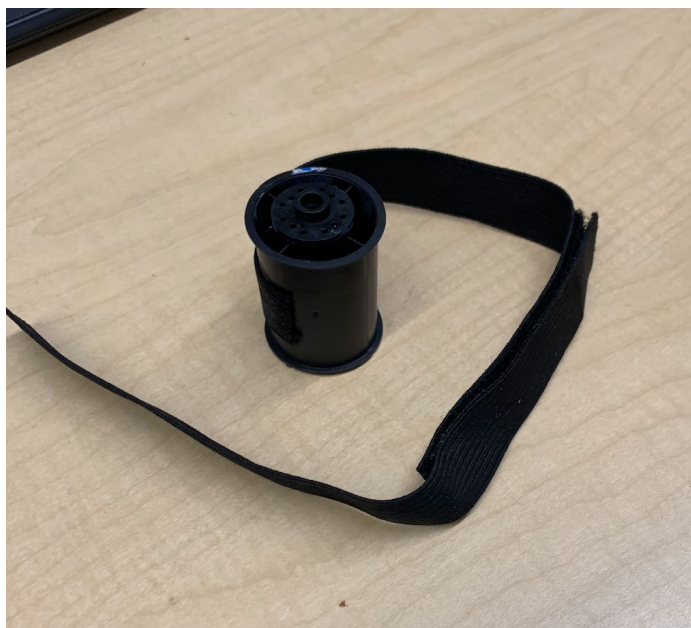
Figure D7: Constricting band connected to the tip of the servo motor.
